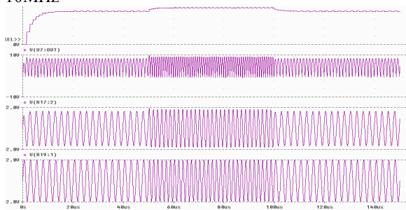
Fig : (4) Output & different waveform of proposed FVC Using S/H technique
